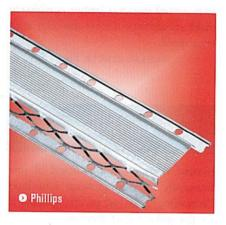
Manufactured with 25 gauge galvanized steel, Phillips RC-2 resilient sound channel features expanded metal for quality sound control and hemmed edges for ease of installation. Channel depth is 1/2".
